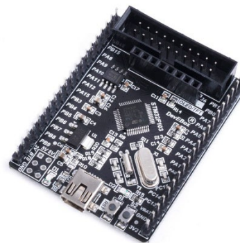
Fig. 6 Appearance of the STM32-Smart microcontroller module.
