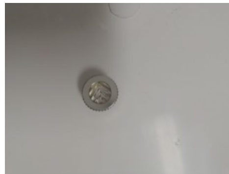
Fig. 2. Cadmium sulfide substrate with dimensions of 5 x 5 x 1 mm 3
