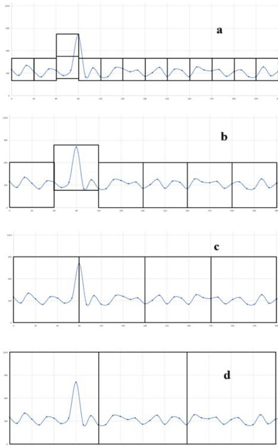
Fig. 4. An example of overlaying on the graph the change in power consumption of a grid with cells of different sizes: a) =30; b) =60; c) =90; d) =120
